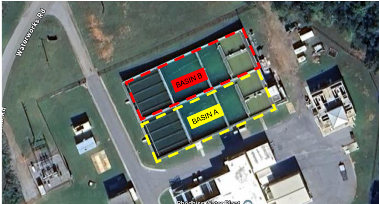
Figure 1. Plan view of the Lenoir WTP Exterior Basins. The Basins are split into 2 sides capable of independent operation. The south side, referenced as Basin “A”, is outlined in yellow. The north side, referenced as Basin “B”, is outlined in red. Basin “A” was evaluated in 2018 along with the Flash Mixer tanks currently under repair.
